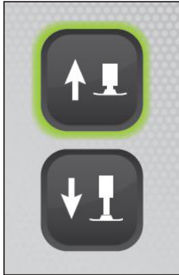
Outrigger Extend / Retract switch
