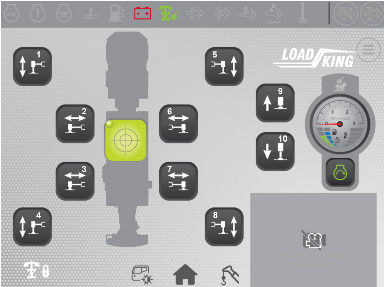
Outrigger controls screen
