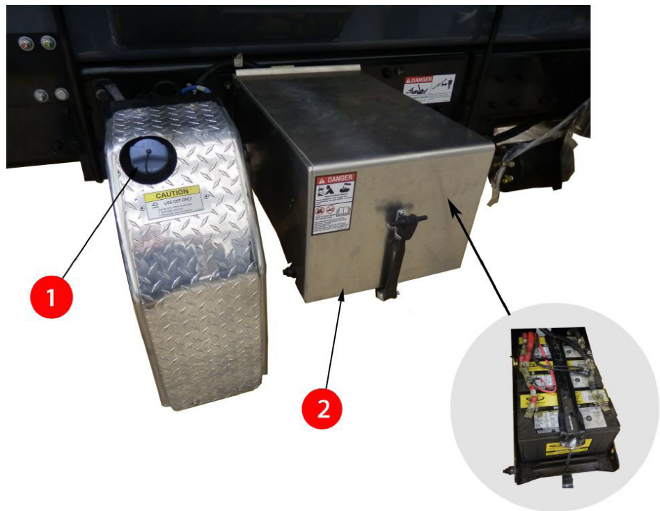
Battery Shelf -Under Left Side of Vehicle
